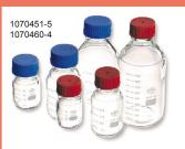
Borosilicate glass with DIN thread GL 45, ISO 4796, graduated, complete with blue or red coloured screw cap and outlet ring. Red coloured screw cap PBTP made incl. PTFE coated seal, heat resistant up to appr. 200°C. blue cap, PP is autoclavable till 140°C. available sizes:
