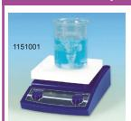
Ceramic plate 180 x 180 mm. temperature till 380 °C, speed 0 - 1,500 rpm, stirring capacity 20 I, heating power 600 W, dimensions 206 x 307 x 99 mm, power AC 220 V, 50/60 Hz.
